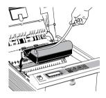
6. Reinstall the image drum cartridge back into the printer, locating the pins on each end into the slots at either side of the printer.
